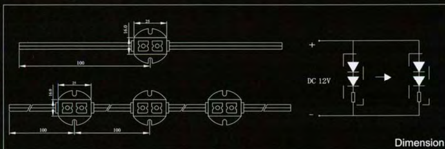
Waterproof 2-LED modules (PVC housing)
