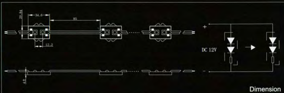
Waterproof 2-LED modules (Aluminium base)
